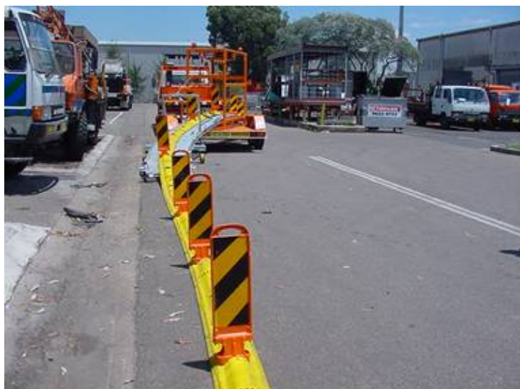
Figure 5.14: A typical movable median unit
