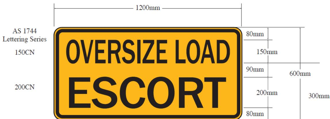
Figure 5 - Escort Vehicle Warning Sign on Vehicle
