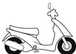
In this example it is obvious that pedalling is not the main means of propulsion. The seat is too low and the pedals are too small and widely spaced to be effective.
