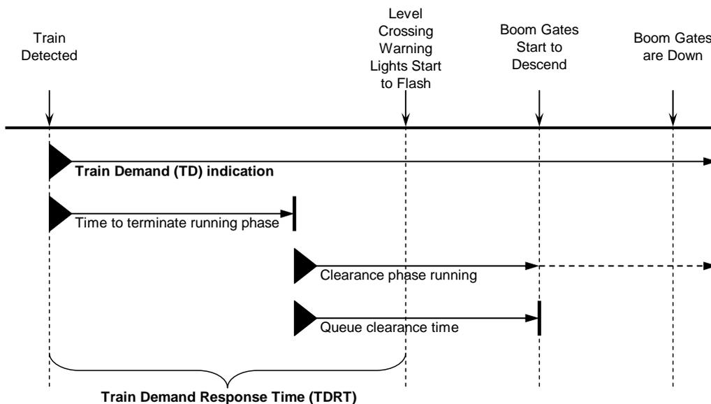
Figure 7 Train demand response time with clearance phase requirement
