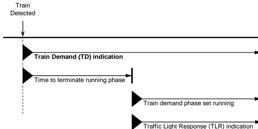
Figure 10 Traffic light response with no clearance phase requirement
