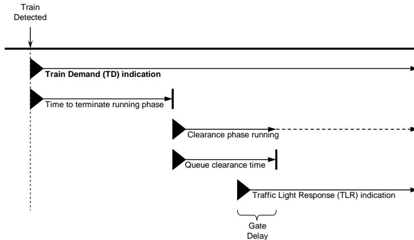
Figure 9 Traffic light response with clearance phase requirement
