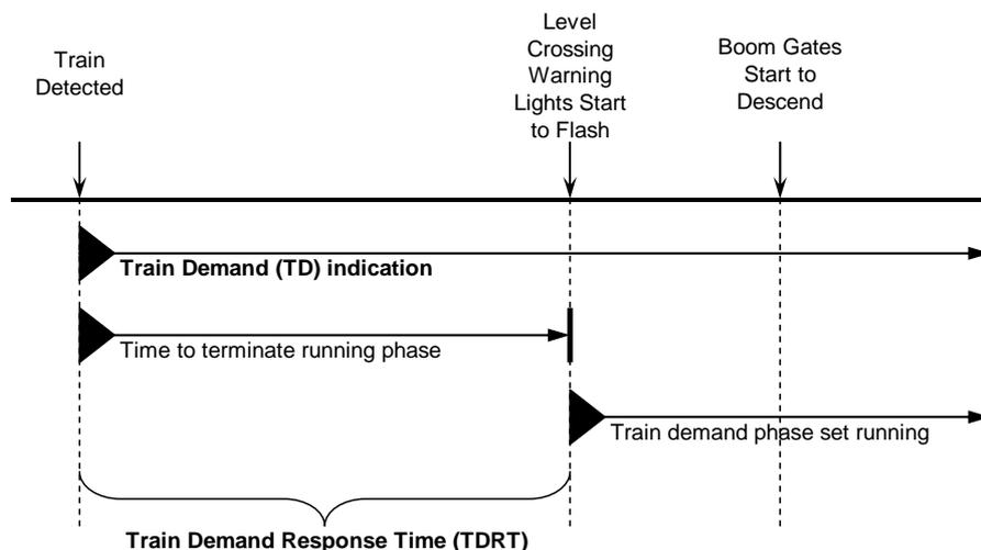
Figure 8 Train demand response time with no clearance phase requirement
