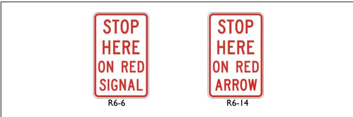
**Figure 10.10 STOP HERE ON RED SIGNAL sign**
