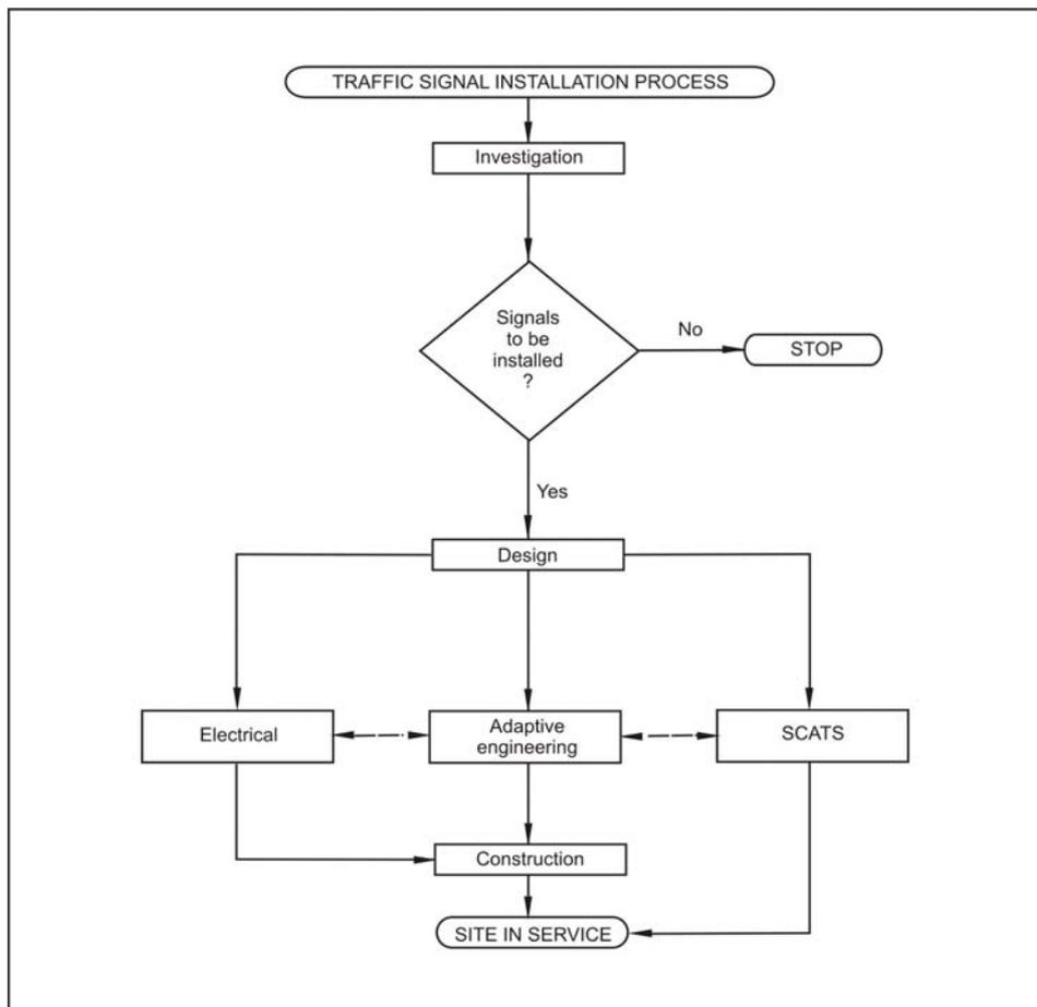
Figure I.1 Stages in the installation process
