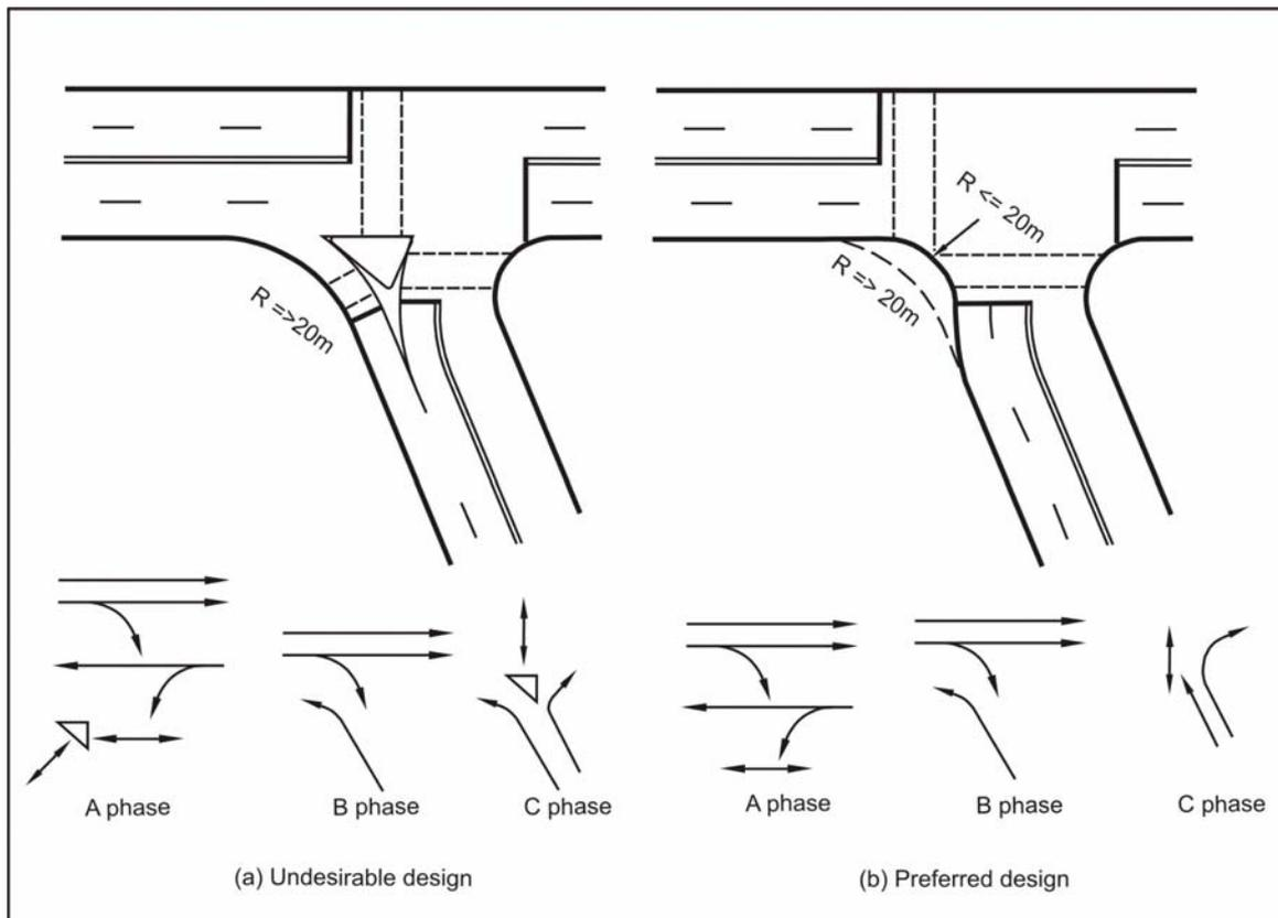
**Figure 5.3 Eliminating corner island to improve design**
