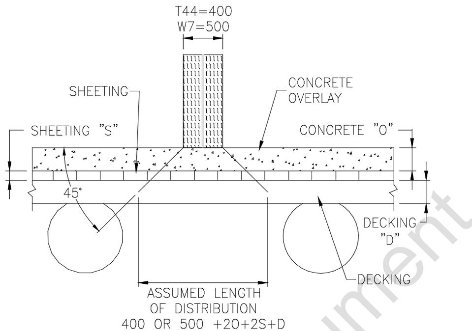
**Figure 6.6.4.3-3 Section B-B from Figure 6.6.4.3-1 – Distribution of Wheel Load Along Deck Planks**
