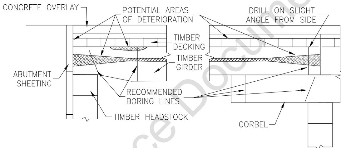
**Figure 6.3.3.4-1 Typical Areas for Deterioration and Boring**
