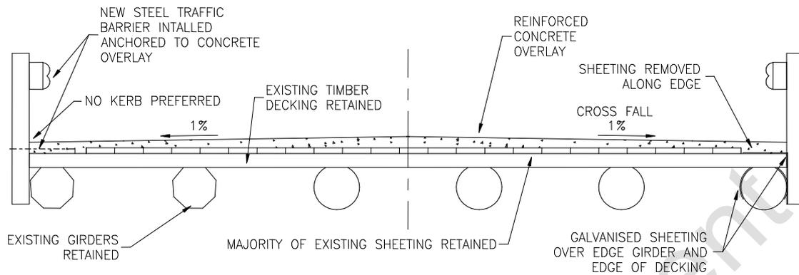
**Figure 6.2.2-1 Traditional Concrete Overlay**
