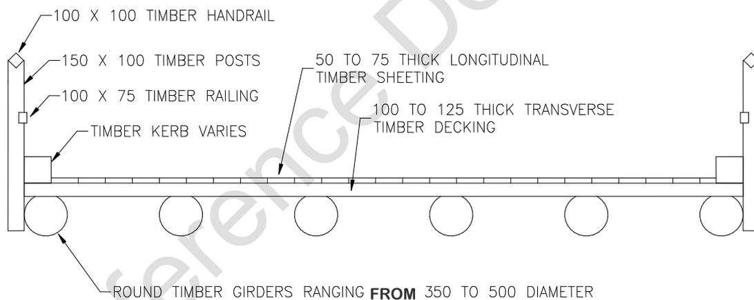
**Figure 6.2.1-2 Cross Section of Typical Timber Girder Bridge**
