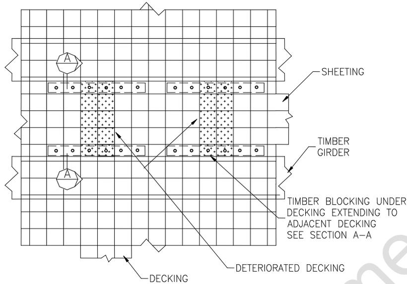
**Figure 6.5.2.2-1 Plan of Decking Repair**
