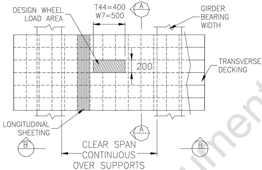
**Figure 6.6.4.3-1 Plan of Design Load on Deck**
