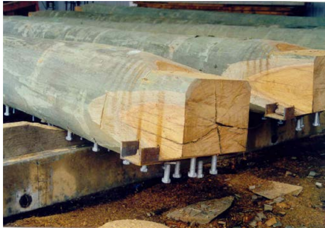
Figure 7.2.2-2 Typical Sizing at End of Timber Girder
