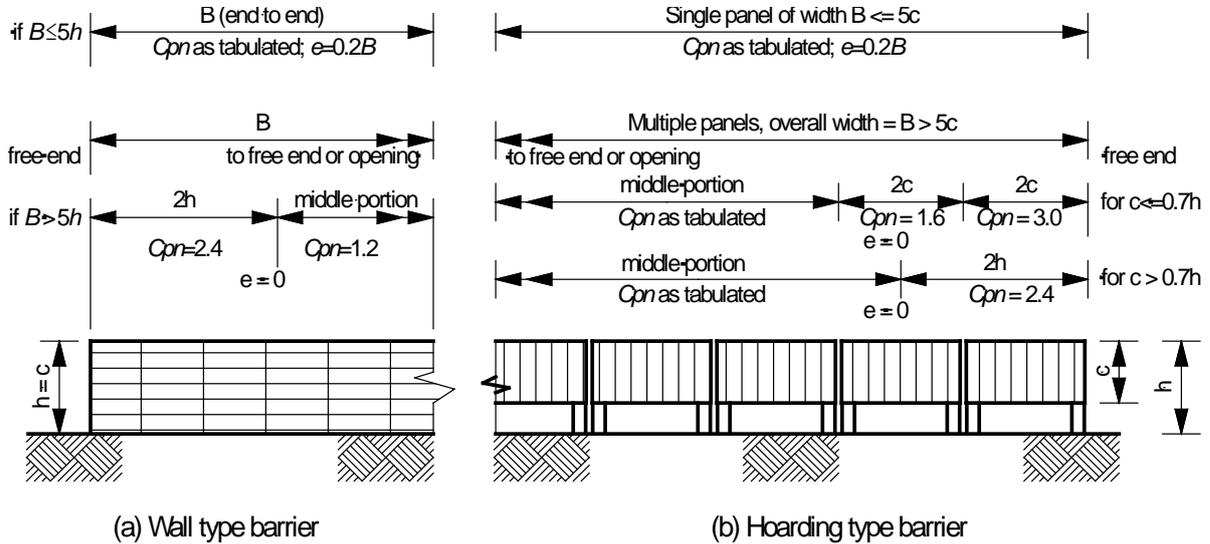
**Figure R271.1 – Wind Pressure Coefficients ( $C_{p,n}$ ) for Noise Walls**
