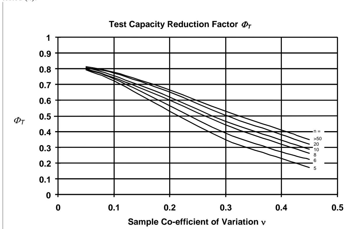
Figure R271/H.1 – Test Capacity Reduction Factor
