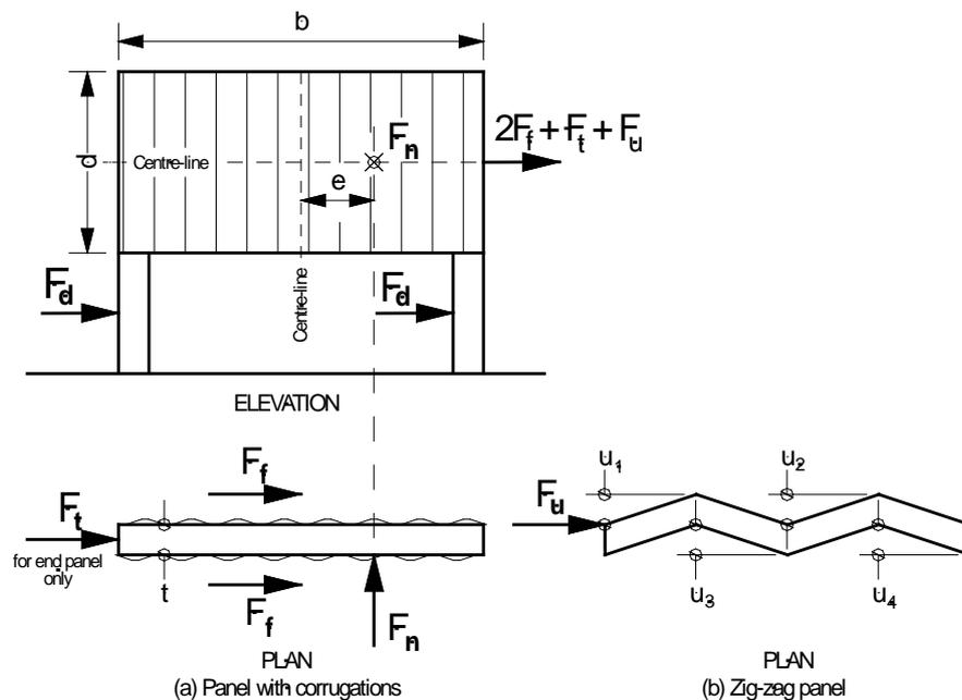
**Figure R271. 2 – Forces on Noise wall due to Wind**
