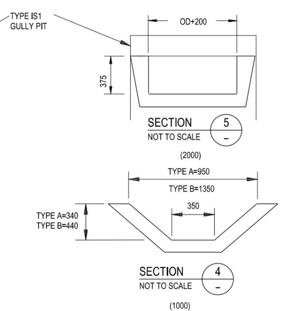
\* INCREASE SIDE OPENING DEPTH TO 450 TO TAKE TRANSITION FROM LINED CATCH DRAINS (TYPES A AND B)
