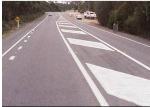
Figure 4.18: Edge Lines (E5) - Outline marking of painted median
