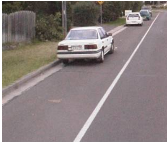
Figure 4.16: Edge Lines (E1) adjacent to moving lanes
