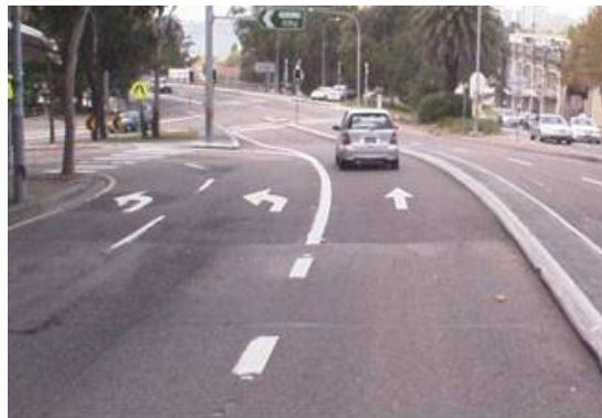
Figure 4.9: Lane Lines (L3) - Discourage lane changing
