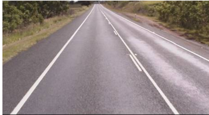
Figure 4.3: Dividing (barrier) line (one-way)
