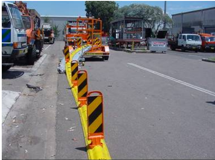
Figure 5.14: A typical movable median unit
