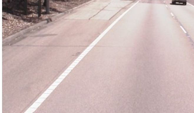
Figure 5.8: Type A Profile linemarking
