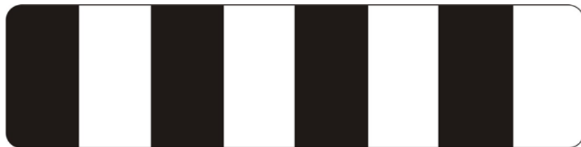
Figure 17.9: Obstruction markers (D4 – 5)
