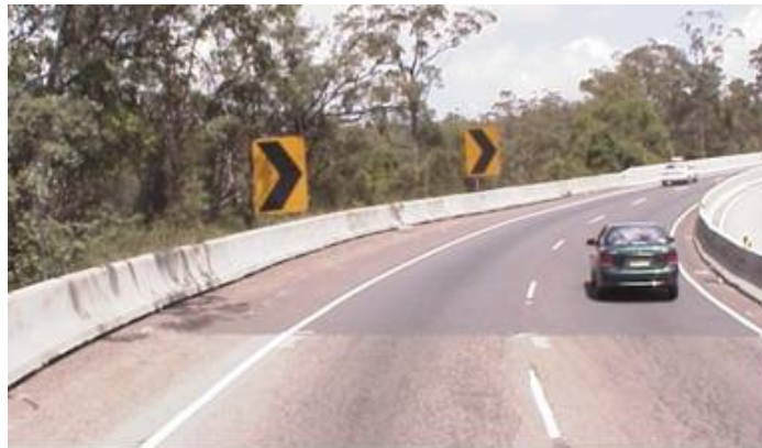
Figure 2.8: Minimum 2 CAMs should be visible at curves
