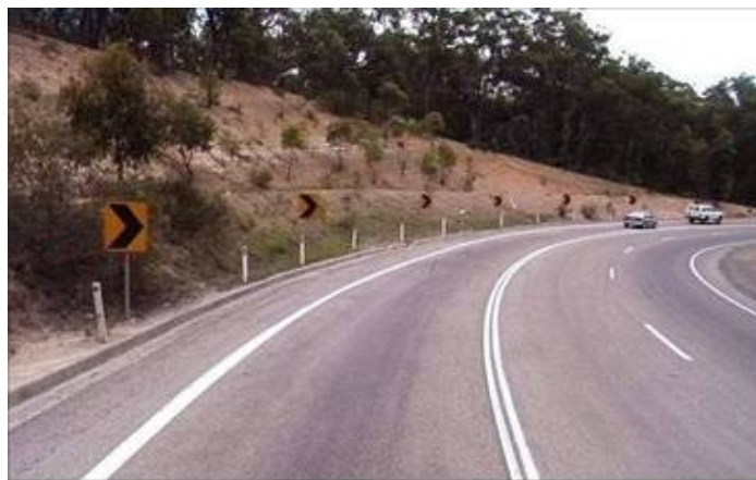
Figure 2.4: Delineation function - conveying road geometry
