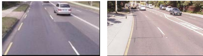
Figure 3.12: Kerbside marking for parking restrictions
