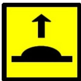
Figure B-12. T5-210 Speed hump ahead sign
