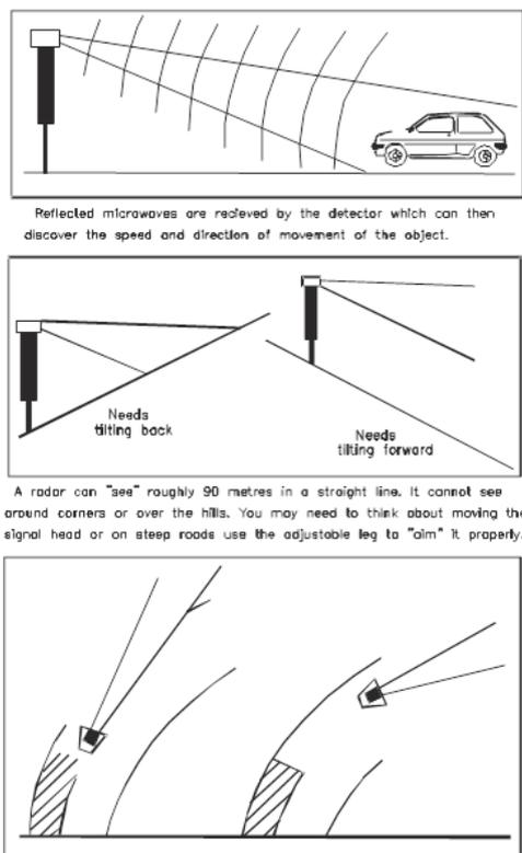
Figure B-2. Illustration of microwave detector operation
