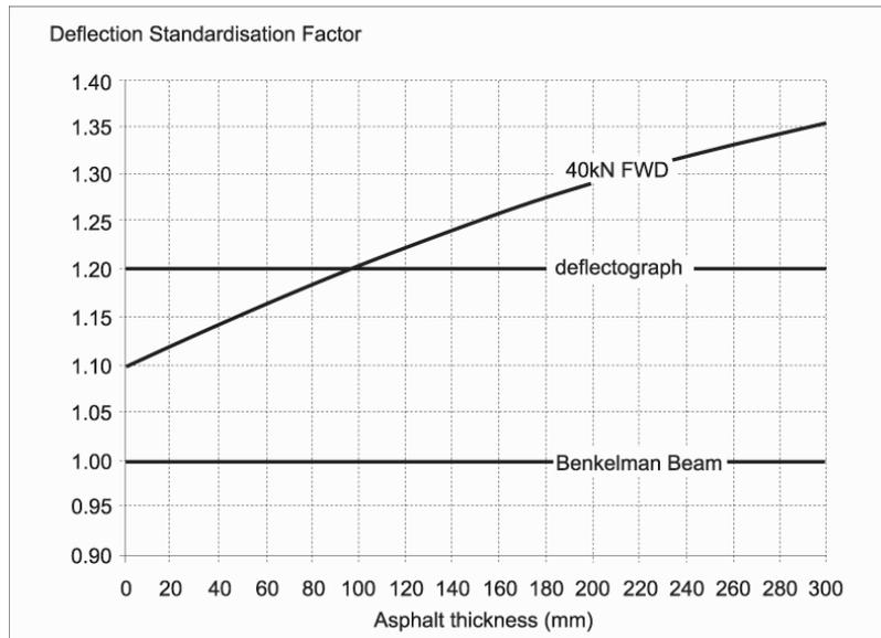
**Figure 12: Conversion factors for the three commonly used deflection methods (Source: Austroads Guide to Pavement Technology, Part 5, Appendix E)**
