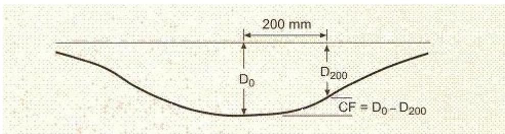
Figure 17: Curvature Function diagram
