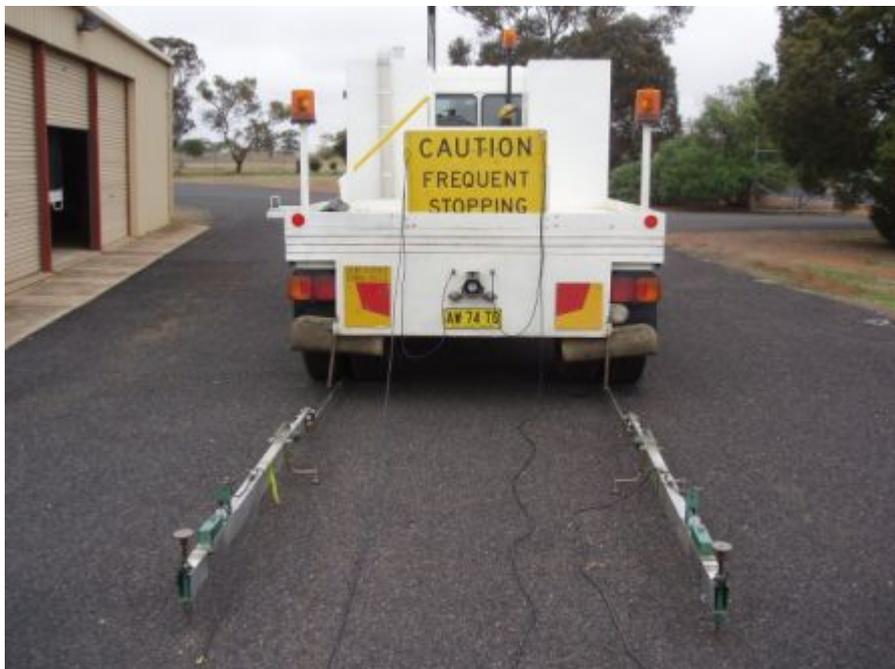
**Figure 9: Example of electronic portable beams extended from the truck**
