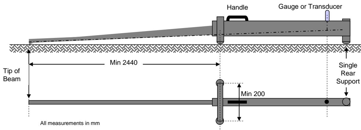
Figure 4: Diagram (elevation & plan) of a typical Benkelman (portable) Beam
