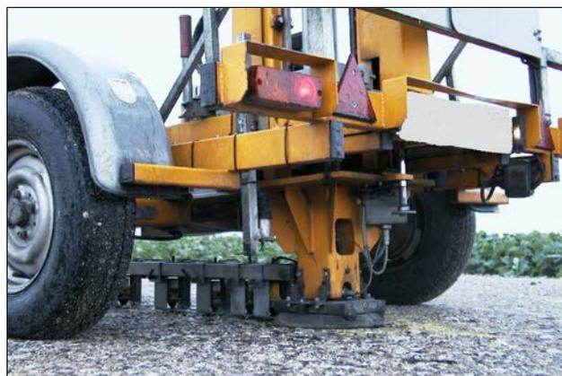
**Figure 3: View of FWD with the geophones lowered onto the road surface**
