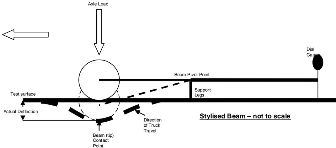
**Figure 5: Schematic diagram of a Portable Beam during operation**
