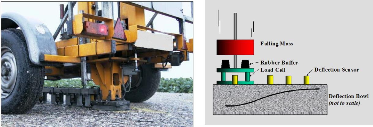
Figure 10: Close up view of the FWD and diagram of deflection bowl
