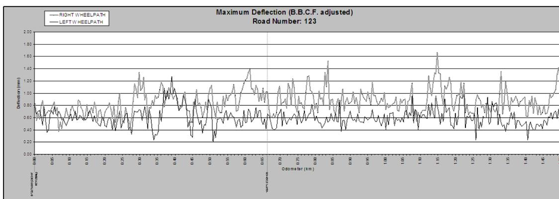
Figure 13: Examples of Deflectograph raw data and associated graph, showing maximum deflection in both wheel paths.
