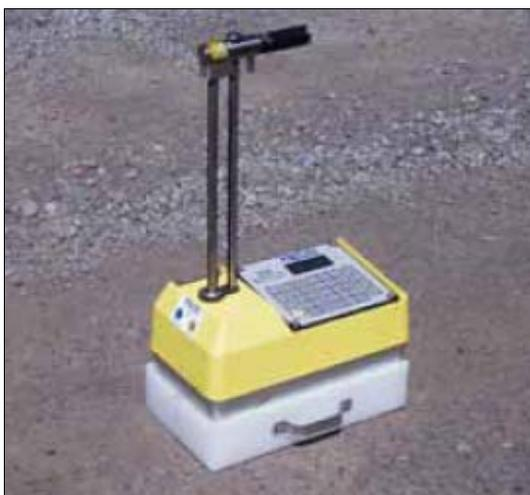
**Figure 1: The NDG is seated on reference block
