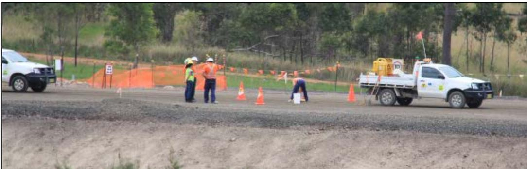
**Figure 3: Staff observing NDG at top of earthworks with safe distance marked out by cones**
