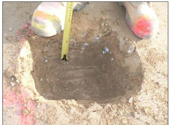
**Figure 8: The material must be taken from the site of the NDG reading (left) and be excavated to the depth of the test**
