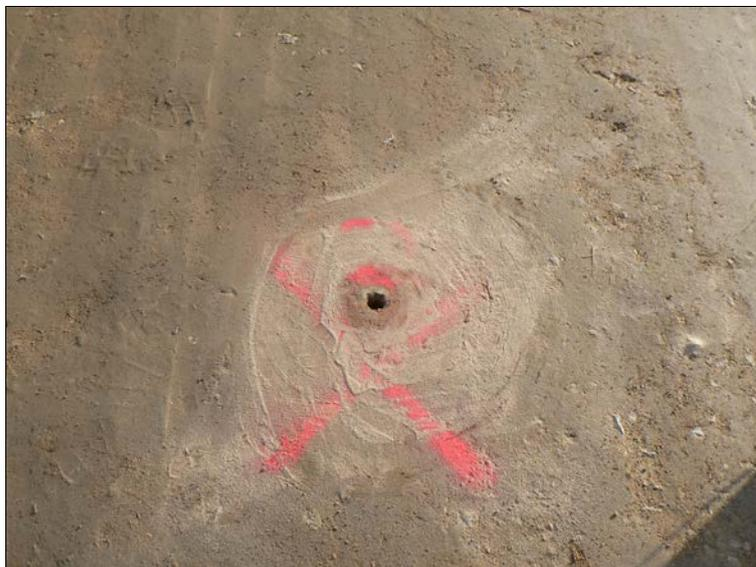
**Figure 6: The site for the NDG must be flat and the hole prepared such that it is circular**
