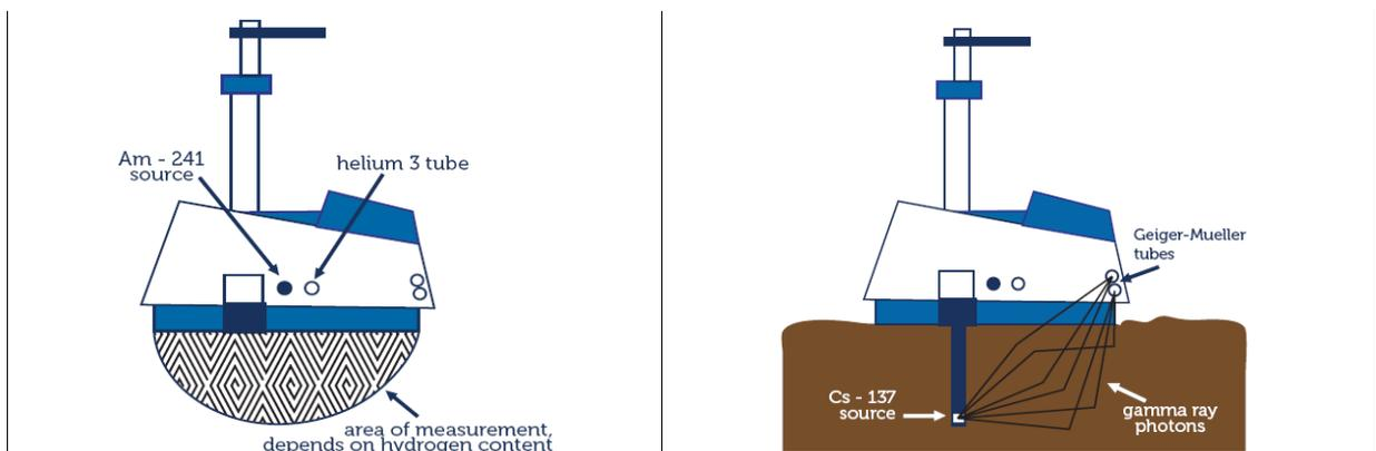
**Figure 5: The NDG operating in indirect transmission (left) and (right) direct transmission mode (Source: APNGA Manual)**
