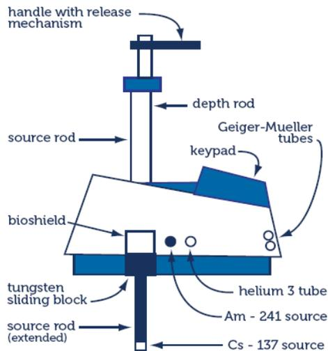
**Figure 4: A diagrammatic representation of the major parts of an NDG (Source: American Portable Nuclear Gauge Association manual)**
