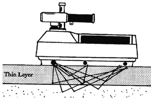
**Figure 9: Thin layer NDG – backscatter gamma paths. (Source: VicRoads TN106)**
