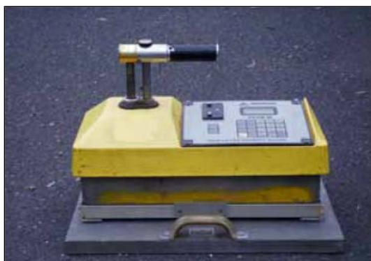
**Figure 2: The NDG Asphalt thin-layer gauge seated on reference plate
