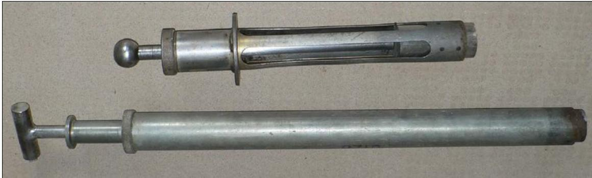
**Figure 3: Standard rammer (top) and a modified rammer.**
