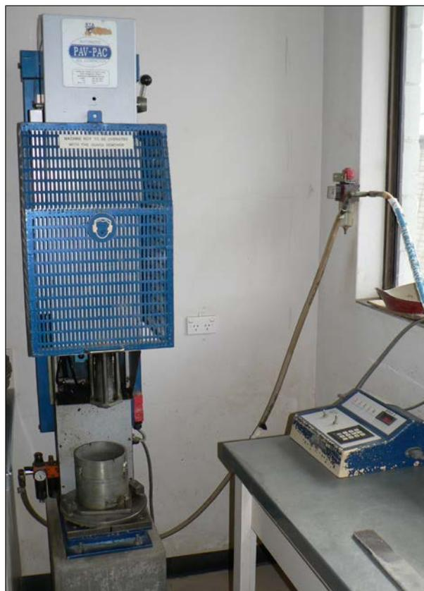
**Figure 4: A typical mechanical rammer**
