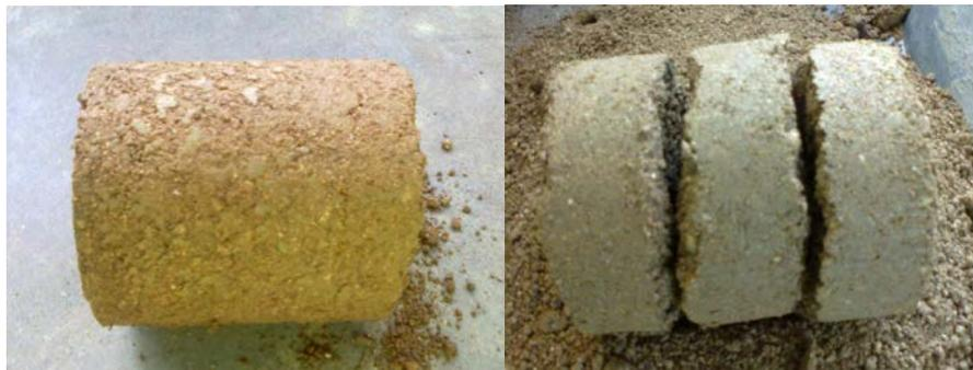
**Figure 5: An extruded compaction specimen and another broken to show three equal layers.**
