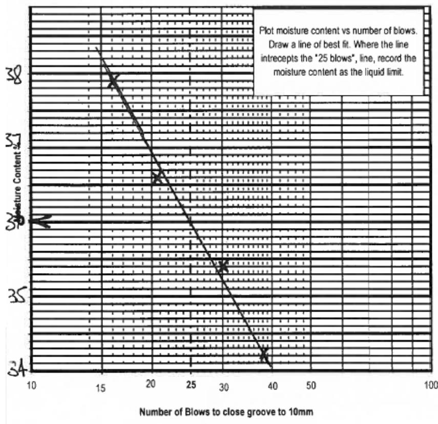
**Figure 10: A plot of the moisture content against the number of blows to close the groove at 10 mm**
