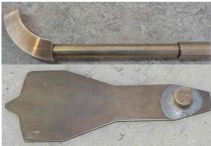
**Figure 4: Two different types of Grooving Tool (left end) and 10 mm Gauge (right end)**
