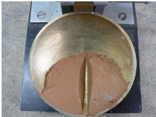
**Figure 7: Liquid Limit material with groove ready for cranking**
