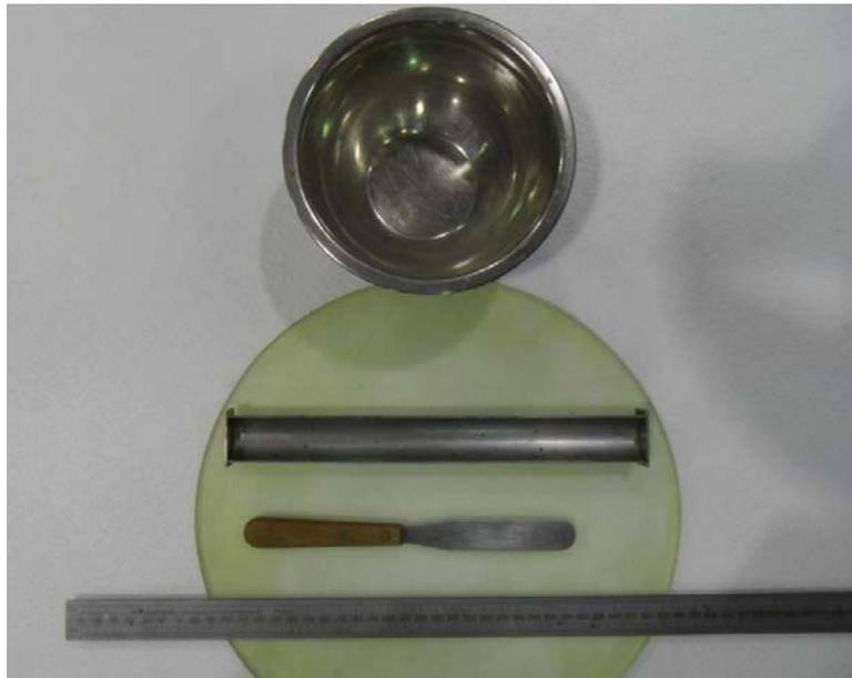
**Figure 14: The shrinkage testing apparatus**
