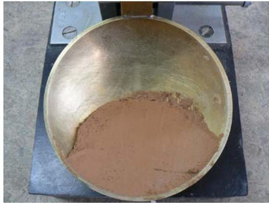
**Figure 6 Liquid Limit material placed in the cup ready for testing.**
