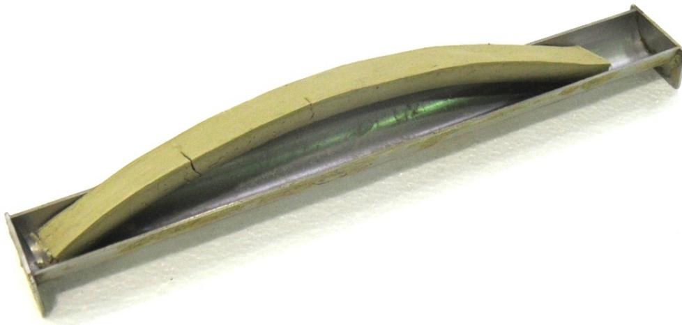
**Figure 17: Dry specimen curled in the mould indicating fast drying**
