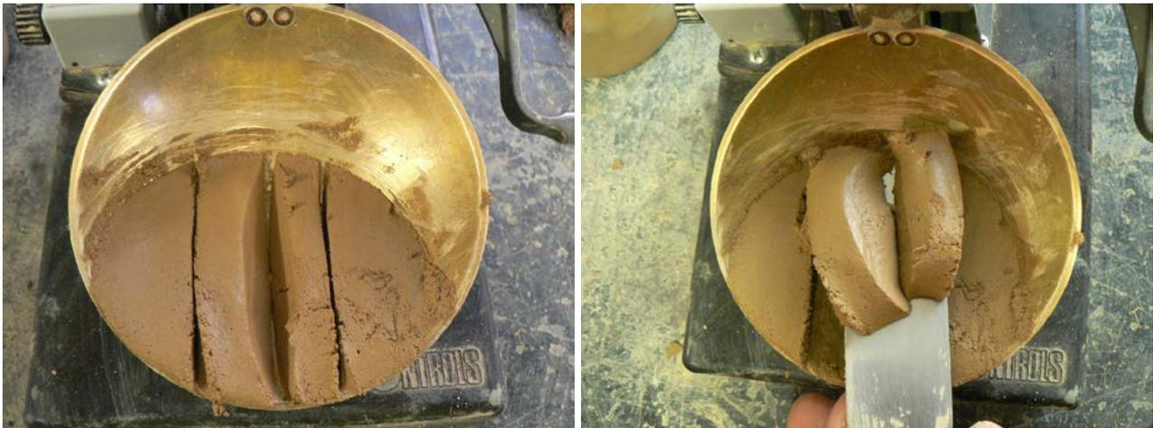
**Figure 9: Taking a representative sample for moisture content**
