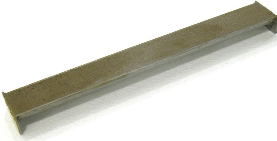
**Figure 15: Wet specimen in mould before drying**
