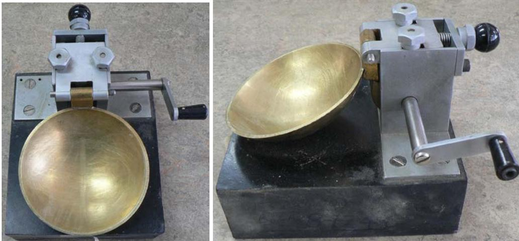
**Figure 3: Liquid Limit (Casagrande) device**
