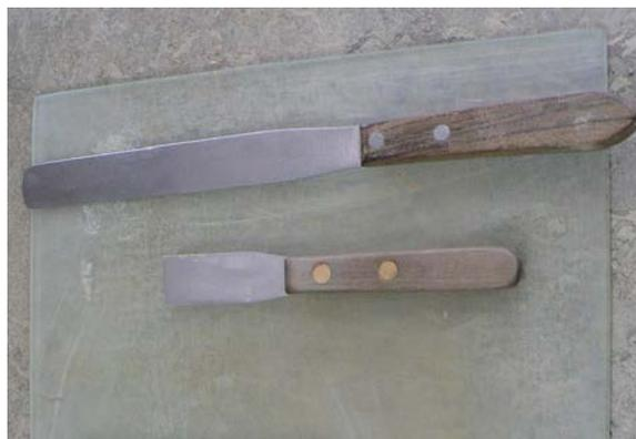
**Figure 1: Glass mixing plate and palette knives**
