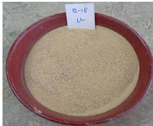
**Figure 5: Liquid Limit material after preparation, now ready for testing**
