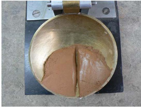
**Figure 8: Liquid Limit material with the groove closed at 10mm**
