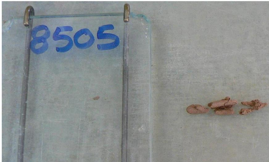
**Figure 13: Material at the Plastic Limit, when crumbled at 3 mm diameter**
