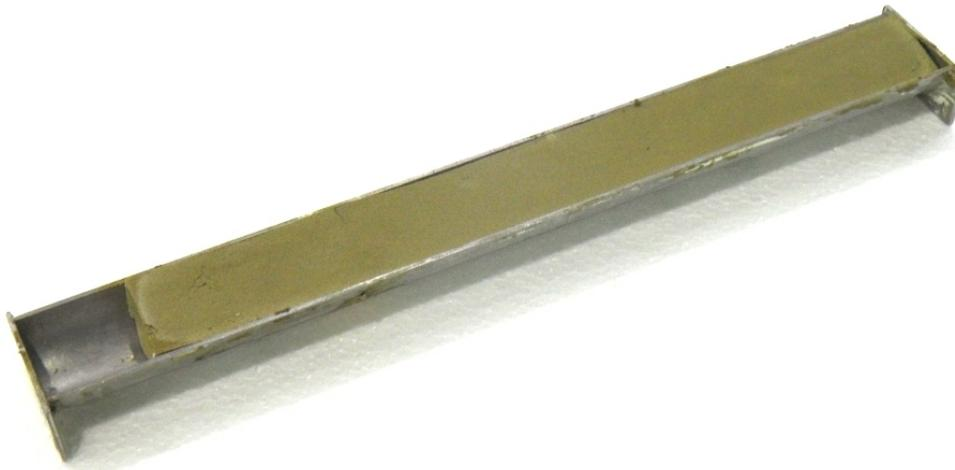
**Figure 16: Dry specimen in mould with a 12% shrinkage value**
