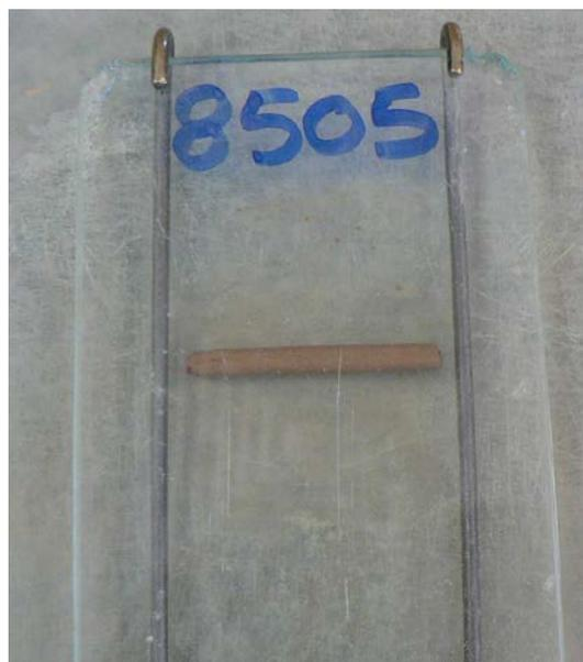
**Figure 12: Material is rolled to 3 mm and in this case the material is still too wet and more kneading and rolling is required**
