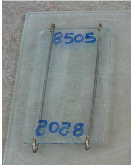
**Figure 11: Glass plate to roll threads and another glass plate with two 3 mm rods used as a 3 mm gauge. (Note the asset number on the glass rolling plate which provides traceability to the calibration checks of the 3 mm rods)**
