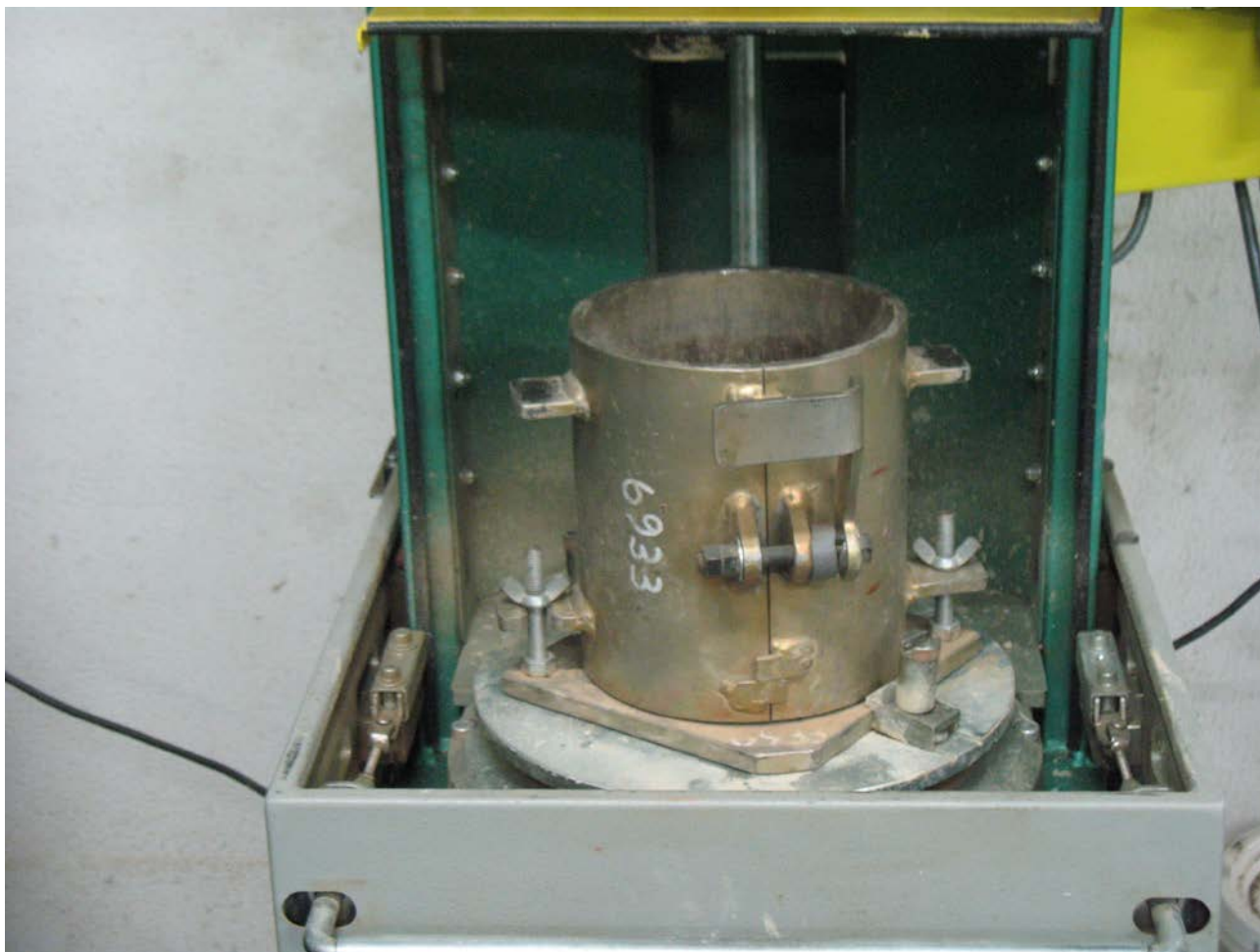
Figure 1: A split mould used for T102
