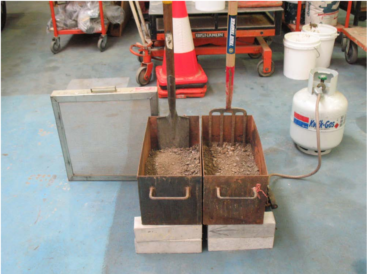
Figure 2: Typical arrangement of soil samples for drying and wetting
