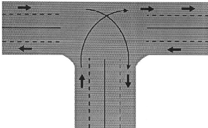
Fig 8. Multi-lane T-Junction into One Way Street
