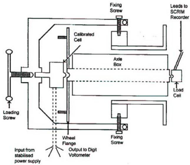
Fig 1. Calibration Jig
