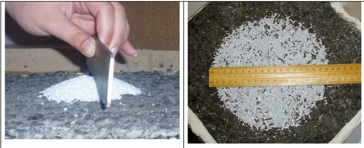
Figure 2-Straightedge placed on peak of cone ready to spread filling material
