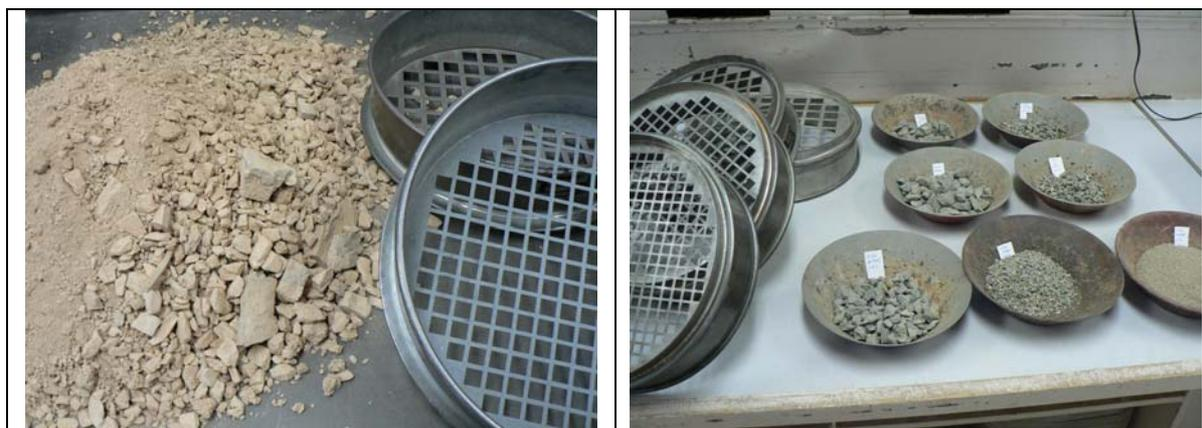
**Figure 1** All pavement and earthwork materials can be grouped into particle size ranges.
