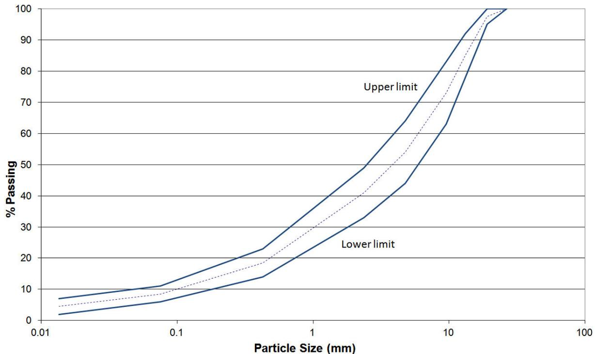
**Figure 3** Grading envelope showing a material (dotted line) that fits the requirements for DGB20 in RMS Specification 3051.
