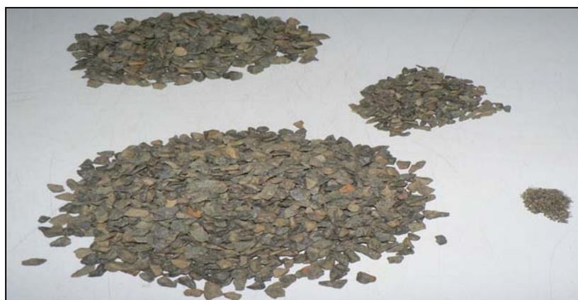
**Figure 10** Aggregate showing the particle size groups after sieving.
