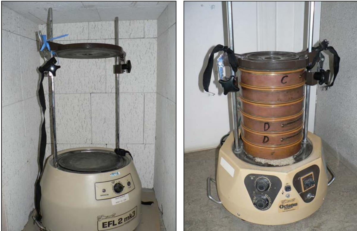
**Figure 6** Typical mechanical sieve shakers used by laboratories.
