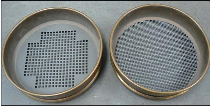
**Figure 5** View of perforated plate (left) and woven wire sieves.
