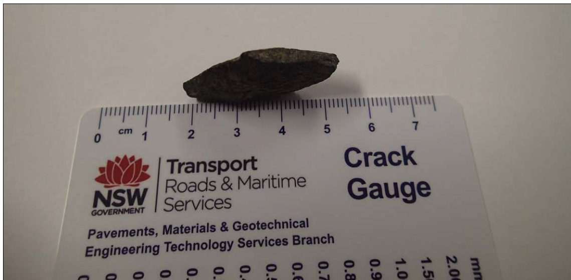
Figure G1: View of crushed flaky aggregate.
