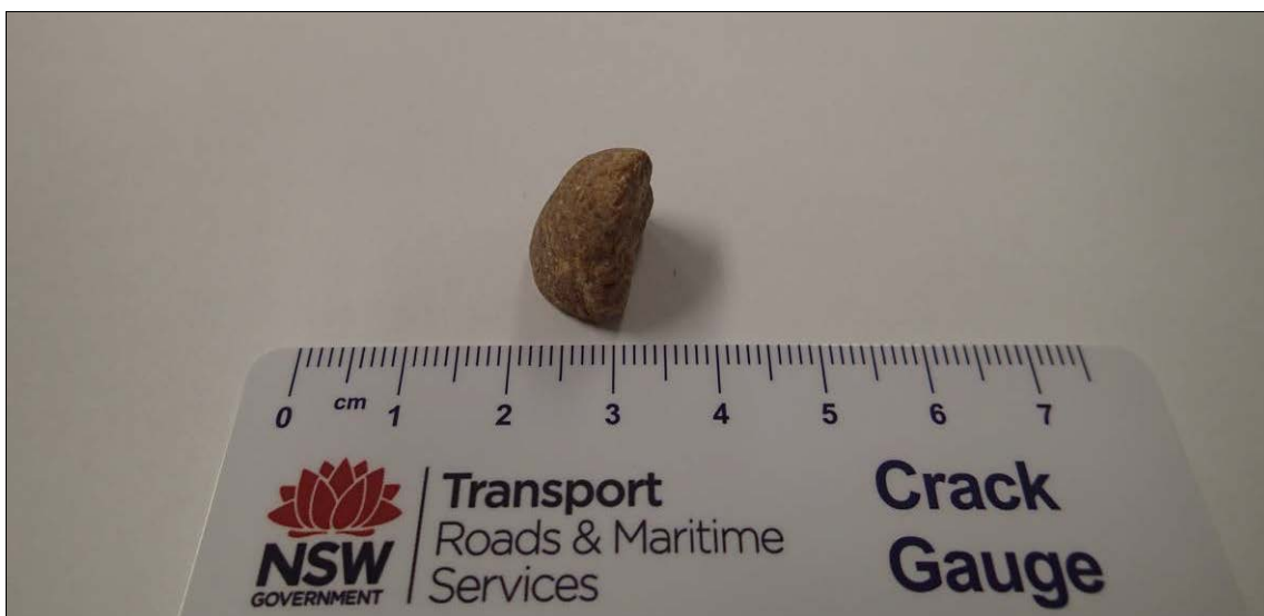
Figure G4: View of partly crushed rounded shaped aggregate.
