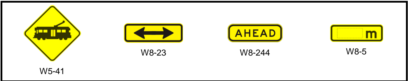
Figure 4. Tram warning sign with possible supplementary plates
