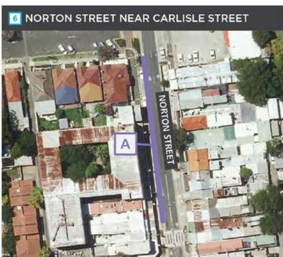
**A** Extend bus zone by about 18 metres to allow for long buses. Remove parking (-3 car parking spaces and -1 motorbike parking space).
