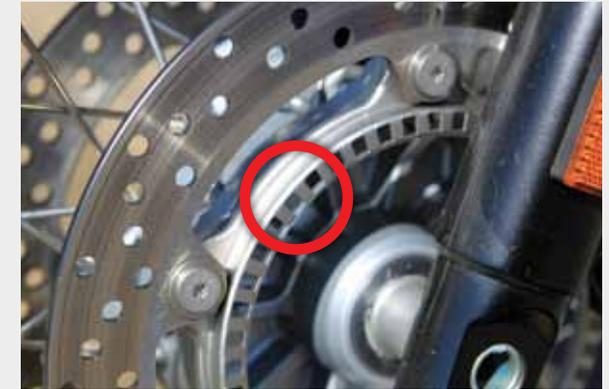
The ABS sensor is an inner perforated ring (circled).
