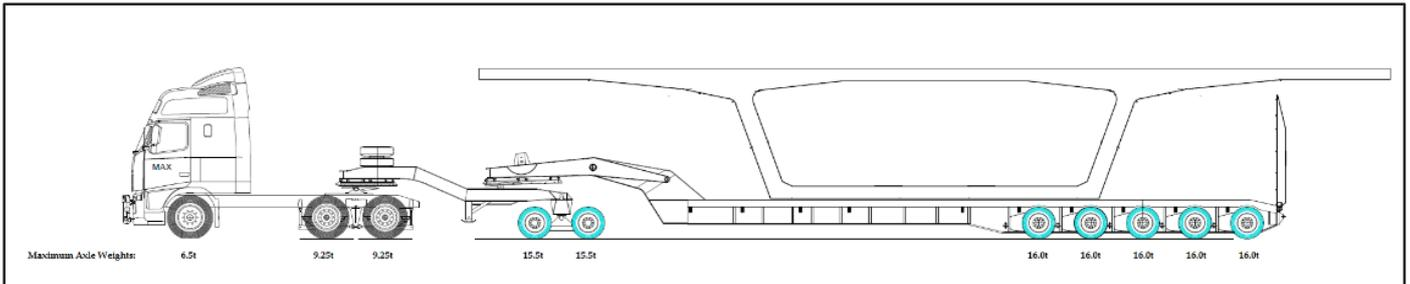
A typical truck used for segment transport. Some of the larger segments will be transported on trucks with more axles.
