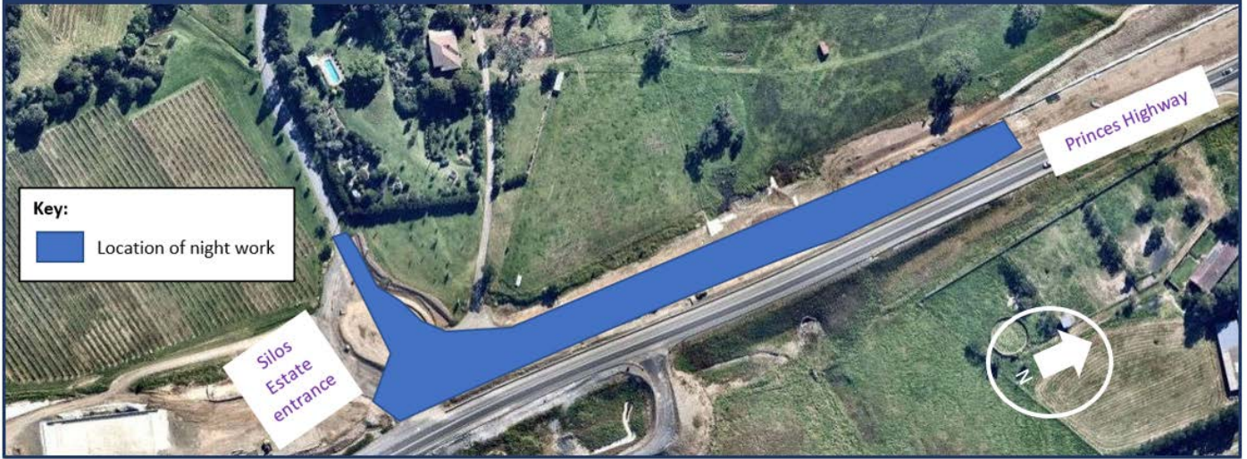
Location of night work for traffic barrier relocation and road line marking removal – Silos Estate entrance
