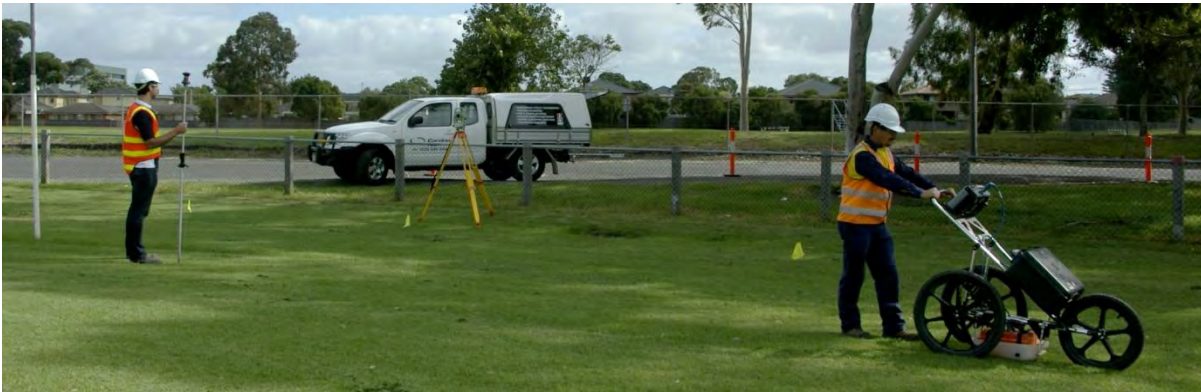
Figure 7-1 Ground penetrating radar with 3D survey location
