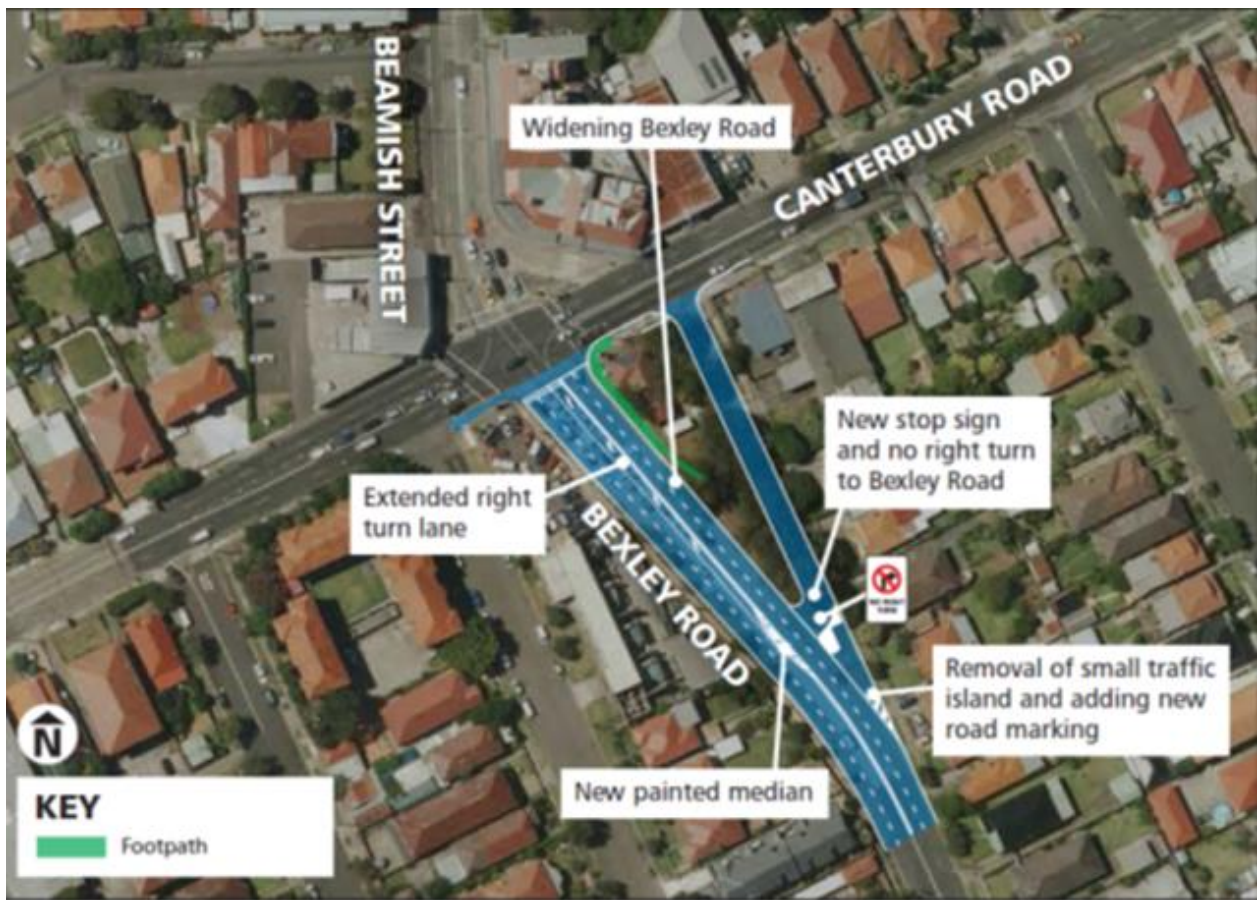
Image one: Proposed improvements on the intersection of Bexley Road and Canterbury Road, Campsie
