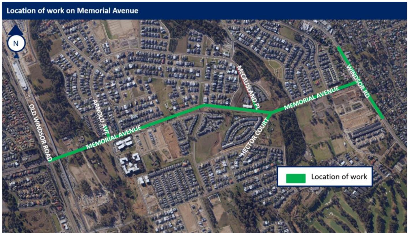
Transport for NSW is upgrading Memorial Avenue from a two lane to a four lane road with the option to expand to six lanes if needed in the future. This will improve traffic flow, ease congestion and reduce travel times along Memorial Avenue and nearby roads especially during the morning and afternoon peaks.
