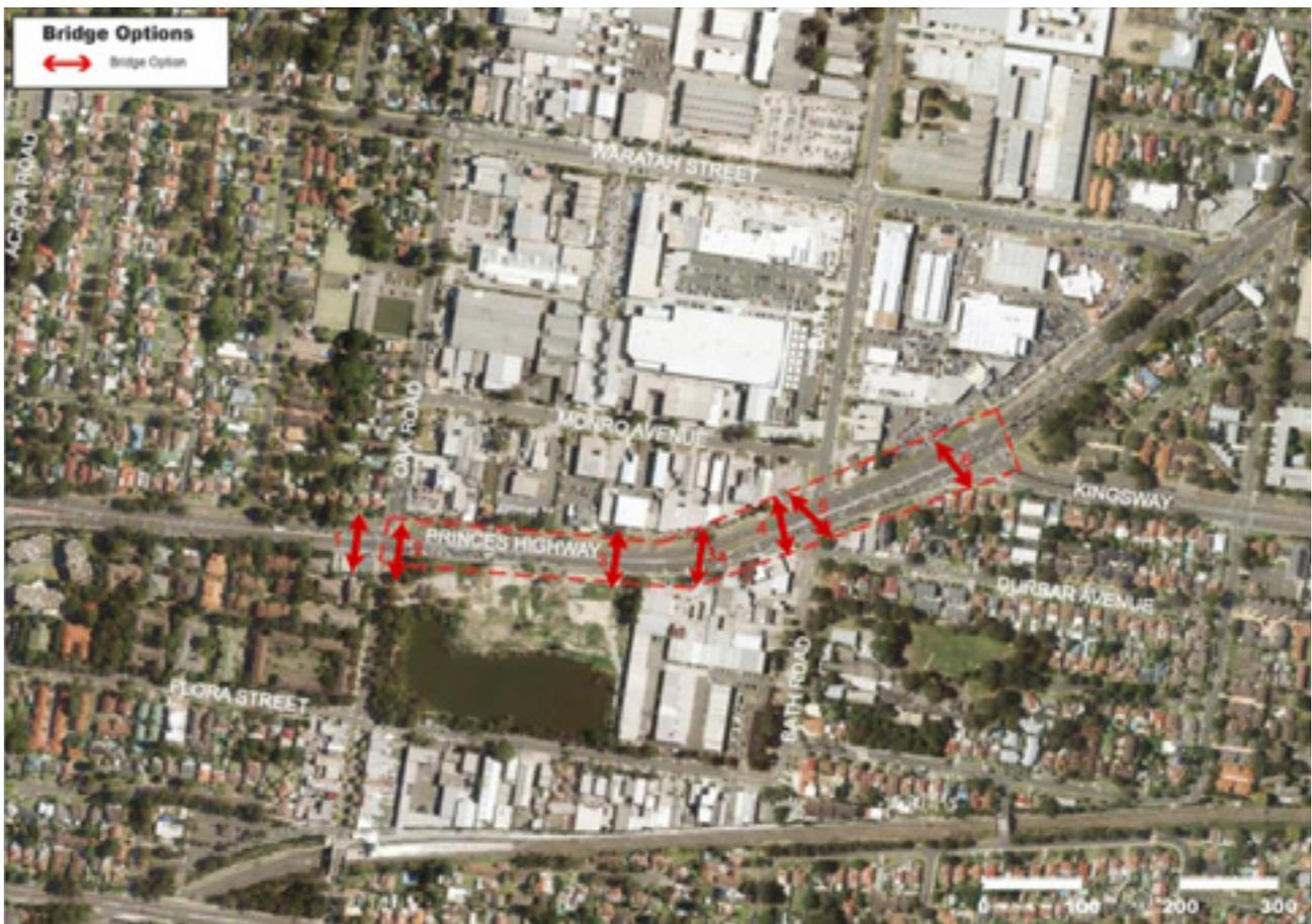
A multi-criteria assessment of each potential location option was undertaken, using the feasibility criteria of TDT2012/05, and a recommended bridge option was determined. This determination considered that 'Option 5', to land the northern side of the bridge adjacent to 530–535 Princes Highway and the southern side of the bridge adjacent to 540 Princes Highway, at the Princes Highway and Bath Road intersection, was the optimal solution.
