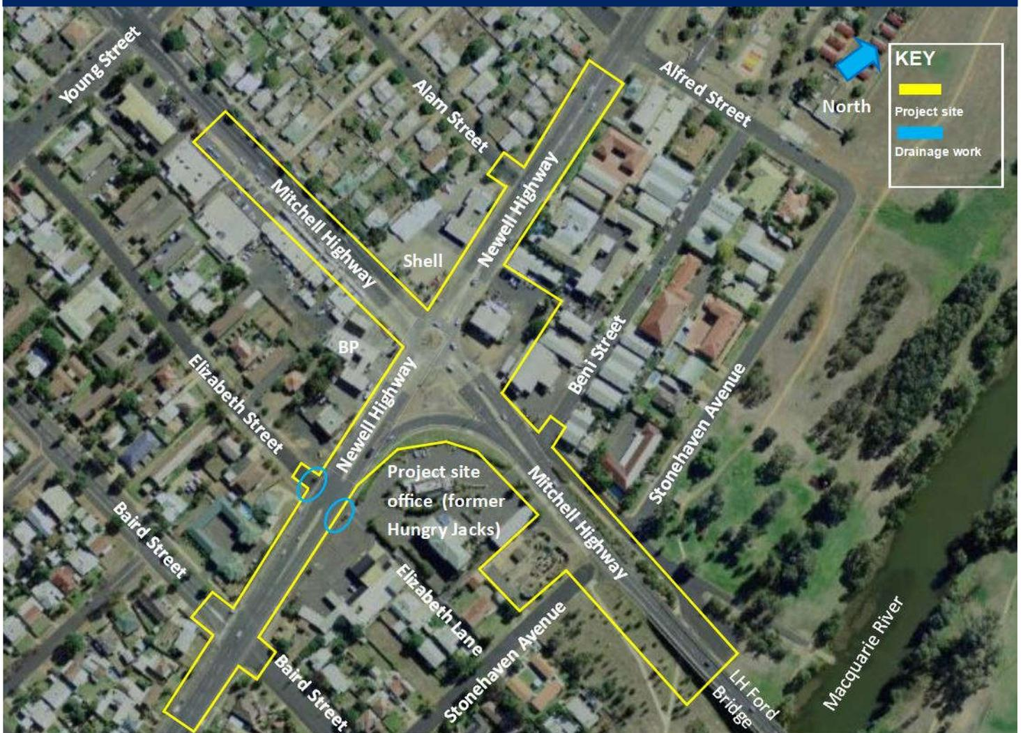
The existing roundabout at the intersection of the Newell Highway and Mitchell Highway will be removed and replaced with traffic lights. The intersection will also be widened as part of the safety improvements.
