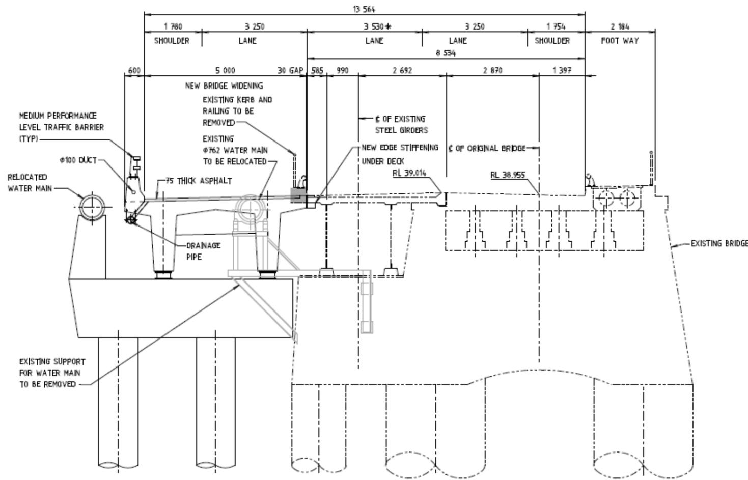
TYPICAL CROSS SECTION AT PIER
