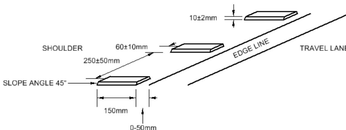
Figure 1 – Specification for installation of white ATLM raised ribs
