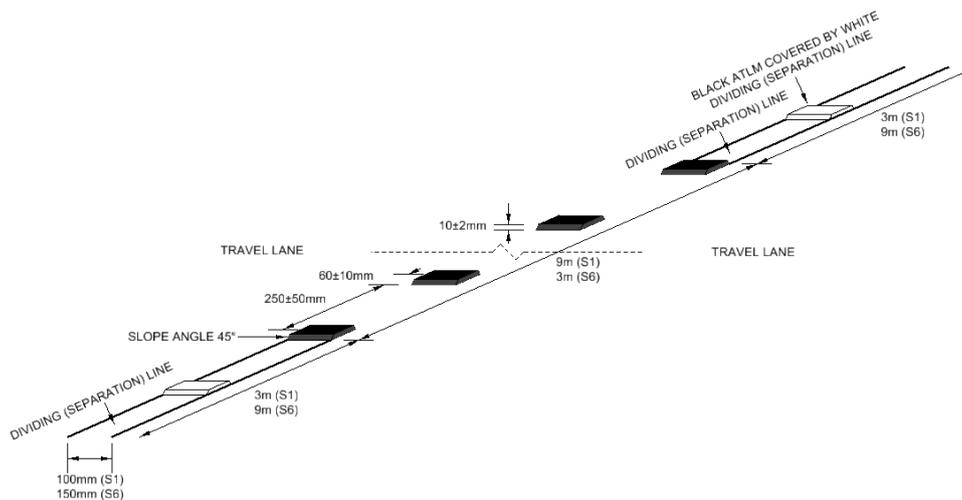
Figure 10 – Black ATLM rib placement for dividing (separation) line treatments
