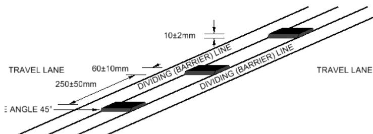
Figure 9 – Black ATLM raised rib placement for standard centreline treatments on rural high speed roads
