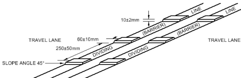
Figure 8 – White ATLM raised rib placement for standard centreline treatments
