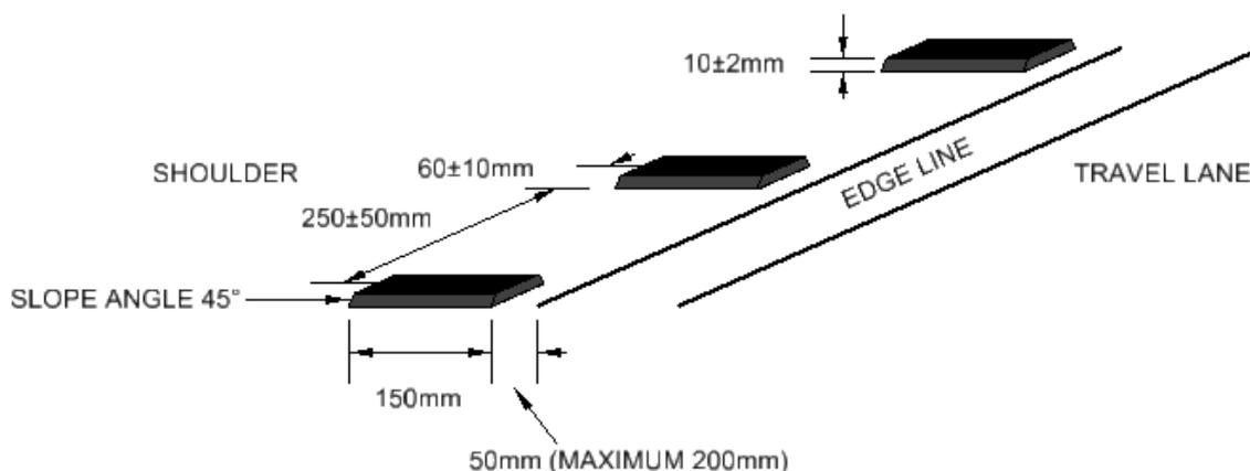
Figure 3 – Specification for installation of black ATLM raised ribs on edge lines
